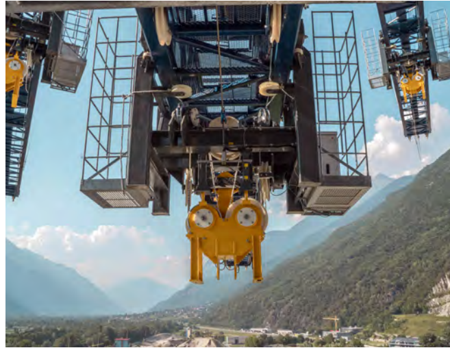
Above: The crane stands 80m over a valley in Ticino. The concept is scalable to a 100m-high tower using up to 8,000 blocks
