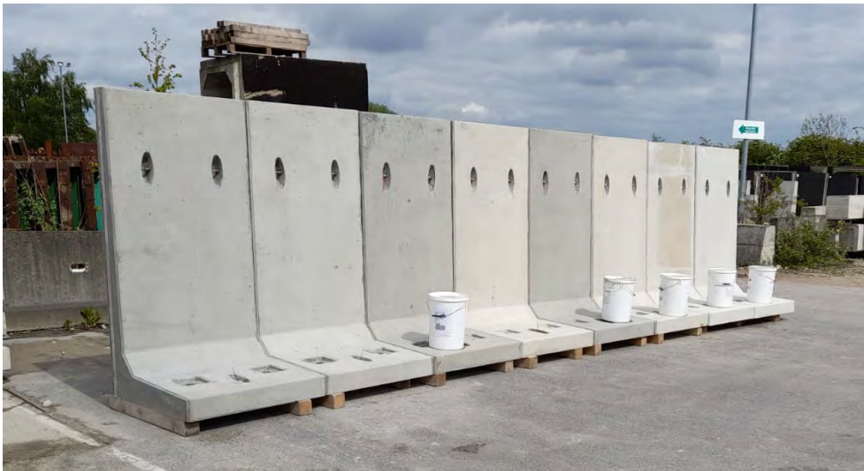
Left: A demonstration precast project by the MPA, trialling the use of limestone powder in multi-component cements
