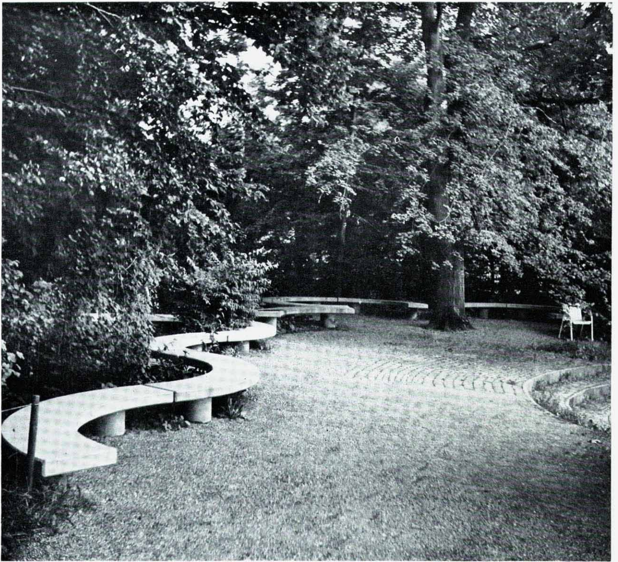
Curved segments of precast concrete form a very satisfactory informal edging to a wooded corner.
