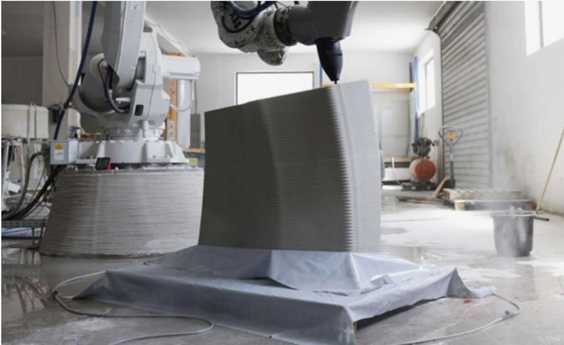
effectiveness of the 3D-printed concrete manufacturing process. Each was formed by up to 500 layers of printed concrete using a two-part mix in which a bead of concrete “ink” is printed together with an accelerator that causes it to set almost immediately.
