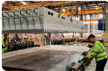
Precast concrete off-site manufacture Assembly building C Bristol by AHMM & PCE Ltd
