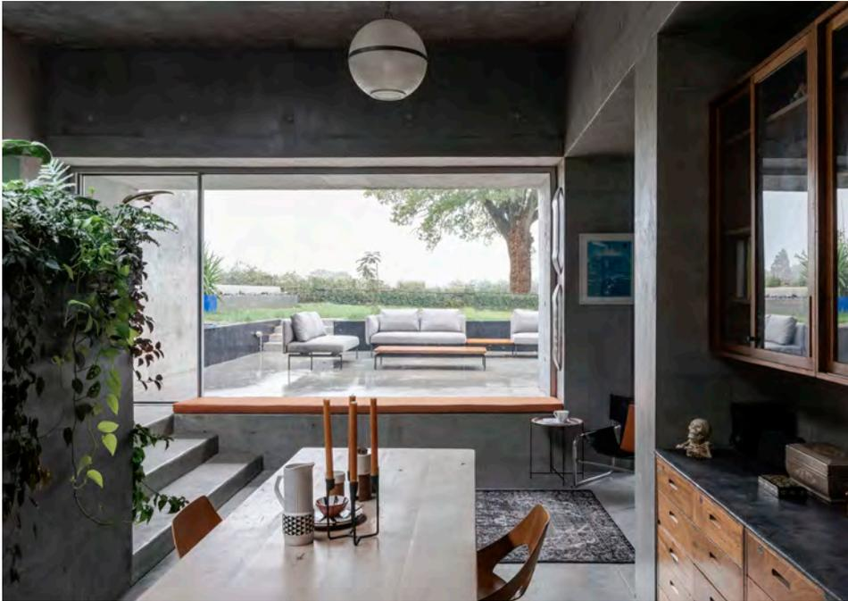
for the slabs, the Resilia HP [High Performance] we supplied for the walls contains a mixture of steel fibres and glass fibres of different lengths. The proportions of steel and glass, together with the different lengths of fibres used, are key to the products' strength."
