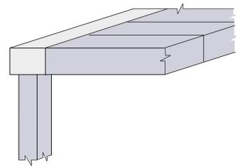
**TYPE 3** Precast column and floor units with in-situ beams
