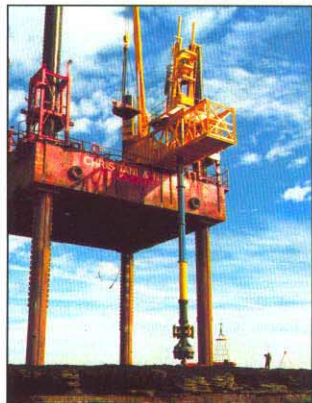
Jack-up at low water with drill-string suspended from the cantilevered drill
