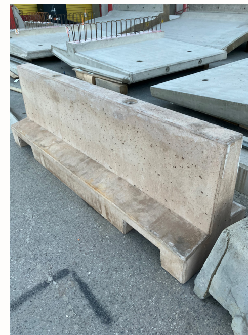
Precast barrier made with calcined clay concrete | EUREKA project
