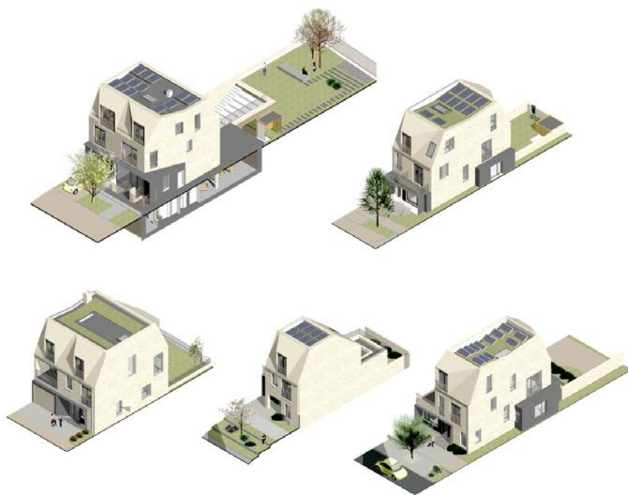
Opposite and right: Knight's Park in north-west Cambridge by Alison Brooks Architects. The all-electric townhouses are part of the Eddington net-zero urban quarter and are formed in traditional loadbearing masonry with precast concrete hollowcore floors. The unusual roof geometry provides different options for solar arrays
