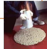
SCC flow test instead of slump test
