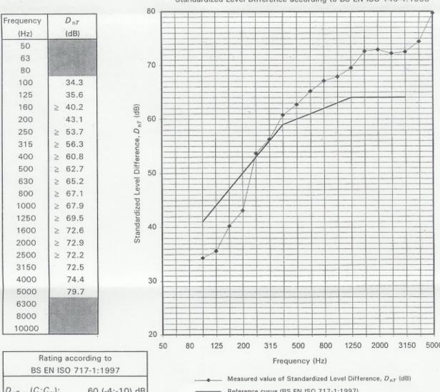
D nT,w (C; Ctr): 60 (-4;-10) dB  $D_{nT,w} + C_{tr} =$ 50 dB
