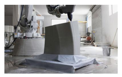
effectiveness of the 3D-printed concrete manufacturing process. Each was formed by up to 500 layers of printed concrete using a two-part mix in which a bead of concrete "ink" is printed together with an accelerator that causes it to set almost immediately.
