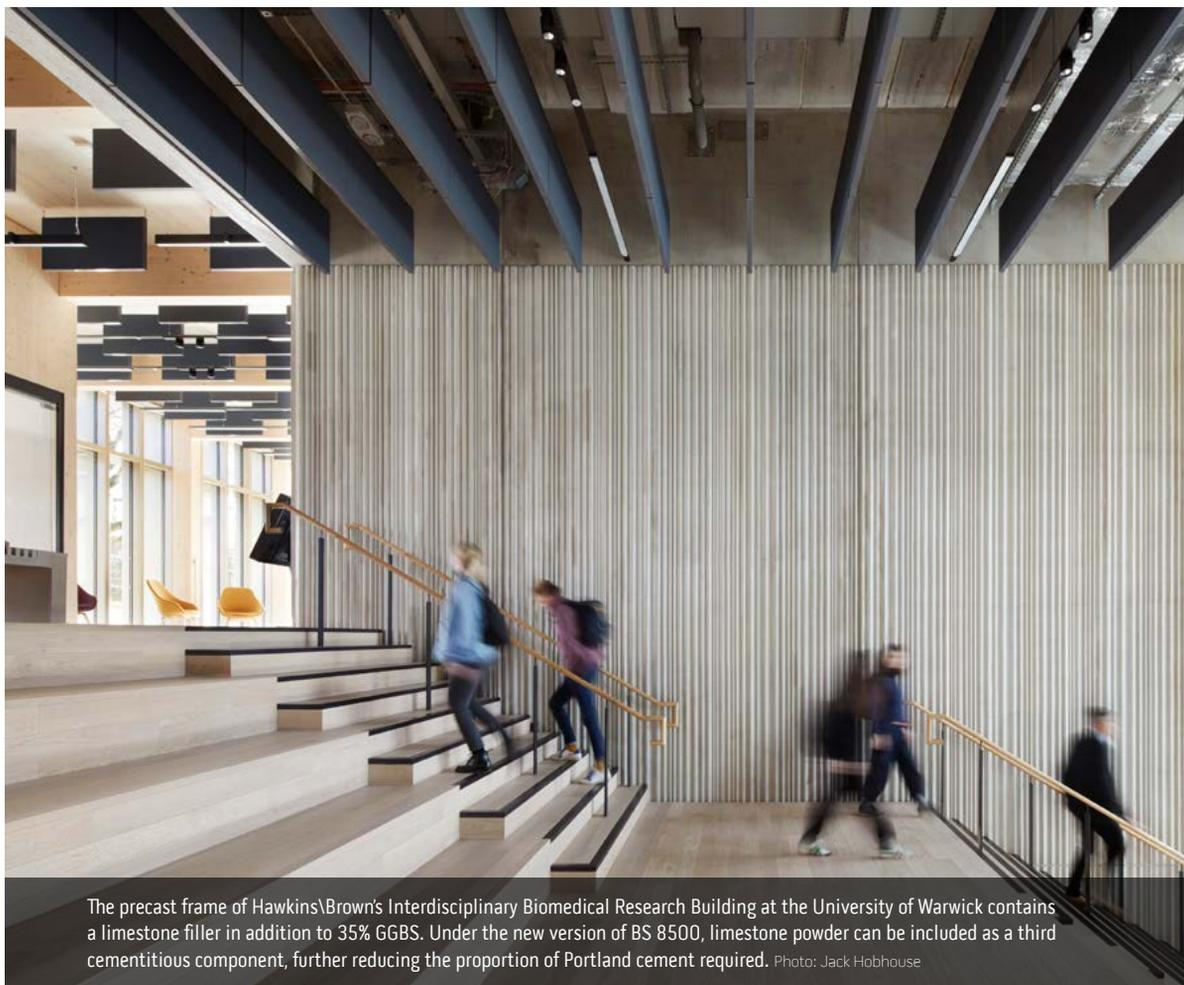
The precast frame of Hawkins\Brown's Interdisciplinary Biomedical Research Building at the University of Warwick contains a limestone filler in addition to 35% GGBS. Under the new version of BS 8500, limestone powder can be included as a third cementitious component, further reducing the proportion of Portland cement required. Photo: Jack Hobhouse
